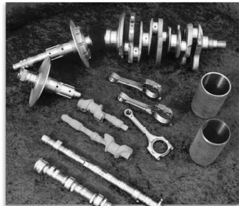
Fig. 2. Family of ferrous products manufactured at the Anna Engine Plant (courtesy of Honda of America)
